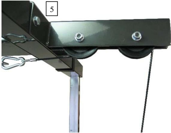
Remove the original upper pulley cable from the machine by taking off the two upper pulleys. The new included Upper Pulley Cable that does not have the black ball stopper will be used for all Upper Pulley work. Replace the pulleys.
