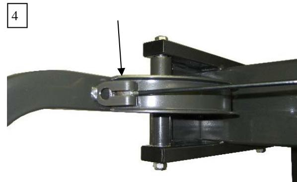
Attach cable to one of the Arm channels and thread the Idler Pulley on the cable before connecting to the other Arm.
