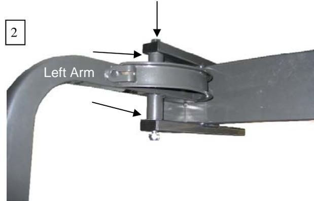
Insert Bearing Flanges on the top and bottom of each Arm and push the Arm into position inside the Bearing Housing frame. Attach with M10 long bolts, washers and lock nuts. Do not over tighten—the Arms should pivot freely.
