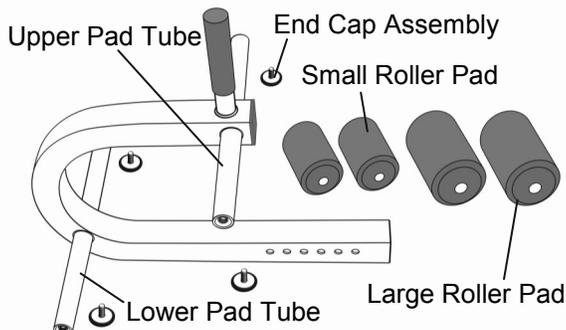
Next, slide the Large and Small Roller Pads into their proper positions. Large pad goes onto the longer Upper Pad Tube and the Small pads fit onto the shorter Lower Pad Tube.
