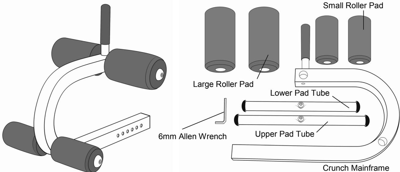
**ASSEMBLY:** Check that all parts are present. Note that Allen Bolts, Round Caps, Flat washers and 4x Black Allen Head bolts are pre-installed on the Upper/Lower pad tubes. With the supplied 6mm Allen Wrench, remove the M12 Allen Head bolts from the middle of the Upper/Lower Pad tubes and all four of the Round Cap/Black Allen Head assemblies. Slide Upper/Lower Pad Tubes into their prospective positions on the Crunch Main frame as shown below and tighten bolts.
