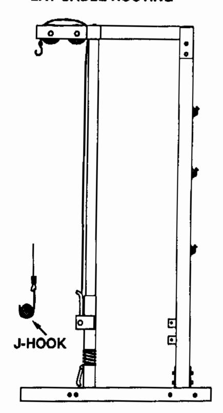
Place Lock Out Pins in the cable position. Hook J-hook on to bar, route cable from behind the back pulley, over the top of both, and then down in front of the front pulley. Attach Lat Bar.
