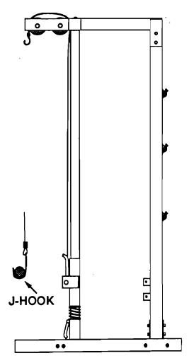
Place Lock Out Pins in the cable position. Hook J-hook on to bar, route cable from behind the back pulley, over the top of both, and then down in front of the front pulley. Attach Lat Bar.
