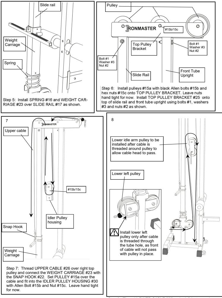
Step 8: Thread LOWER CABLE #27 under left bottom pul-
