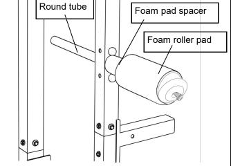
**Step 4:** Install ROUND TUBE #18 using bolt #5 and washer #3. Push FOAM PAD SPACERS #14 on first then the FOAM ROLLER PADS #13. Secure with bolt #7, dome cap #12 and washer #8 as shown in exploded view. Note: There are 3 height positions available so you can select the most comfortable height for the leg hold down.
