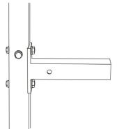
Once the PULL PIN snaps into the stub hole, tighten the PULL PIN to the locked position and make any necessary adjustments to seat height or leveling using the methods show on previous page.
